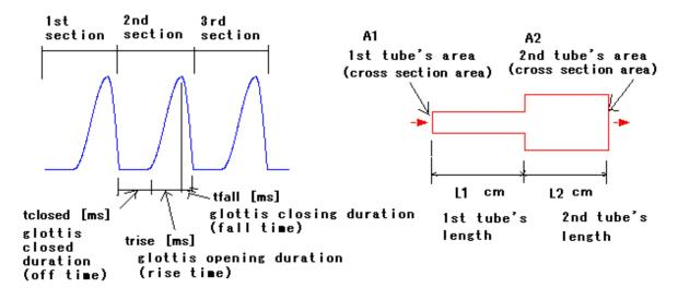
As glottal regulation, closed duration, opening duration, and closing duration can be set. Sum of these three duration relates to pitch period. If pitch period is short, you will hear higher tone sound, contrariwise period long, lower tone. Repeating close and open of glottis, air flow volume velocity is uncontinuous, showing blue color waveform in the left figure above.
